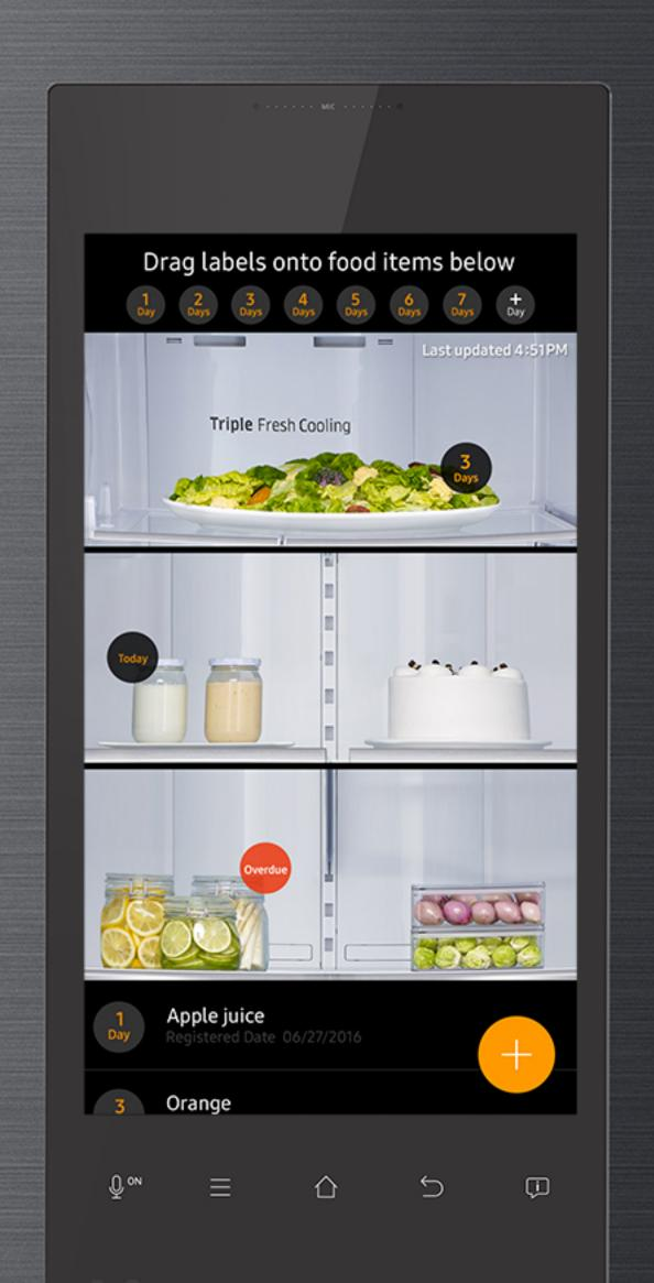
When you close the fridge, three cameras installed in the interior take a snapshot, which is and automatically sent or updated to your smart device.
